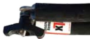
**11.** Replace lock washer and wing nut and slightly tighten.
